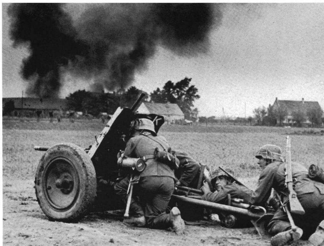
ABOVE: The crew of a 3.7cm Pak 35/36 hunch behind the shield of the gun. The anti-tank gun had a range of 700m (763yds) in action firing a 680g (1 \frac{1}{2} lb) shell.
