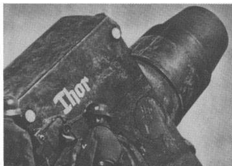
ABOVE: The 5m (16ft 3in) barrel of the 60cm mortar "Thor".
