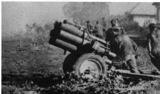
LEFT AND ABOVE: The loading and firing sequence of a 15cm Nebelwerfer – smoke thrower – multi-barrelled rocket launcher. It was developed at the rocket research establishment at Kummersdorf in the 1930s when Germany was banned from building heavy artillery by the Treaty of Versailles. The rocket had a 2.83kg (5.70lb) HE warhead and a maximum range of 7,060m (7,725 yards).
