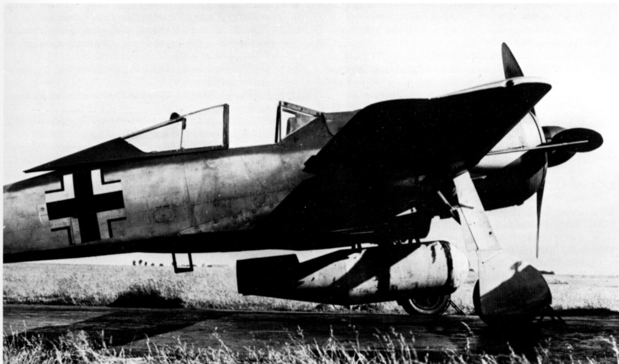
Fw 190A-5 (Werknummer 1286) fighter-bomber, with an SB 1000 rack and 1000-kg bomb.
