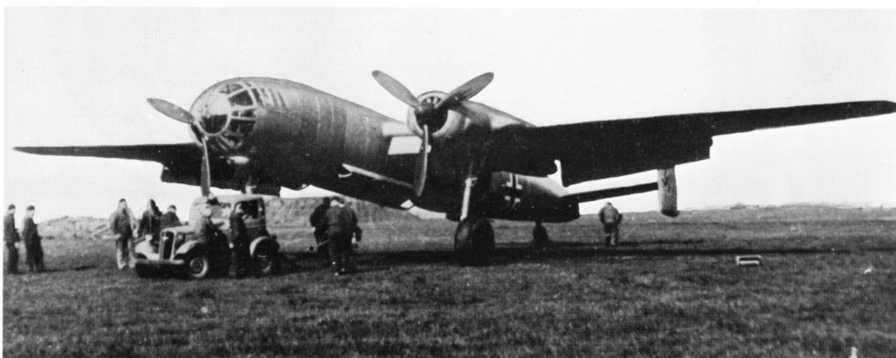
Fw 191 VI with its Multhopp landing flaps fully extended. At this setting, the flaps served as dive brakes.
