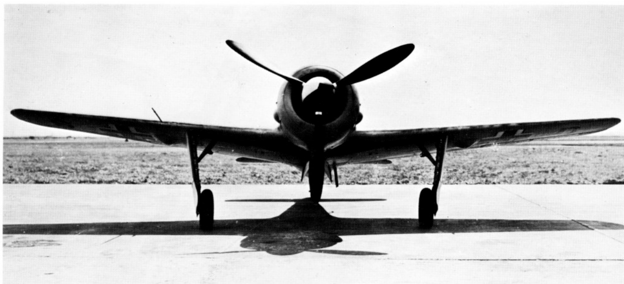
Fw 190A-1, 1941, fitted with the BMW 801C, an engine rated at 1147 kW/1560 hp.
