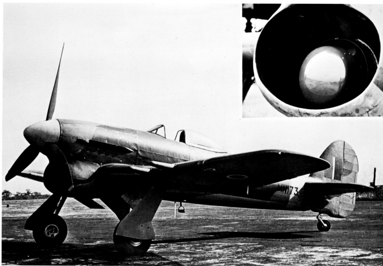
Hawker Typhoon IB with 24-cylinder Napier Sabre IIA, rated at 1602 kW/2180 hp.
