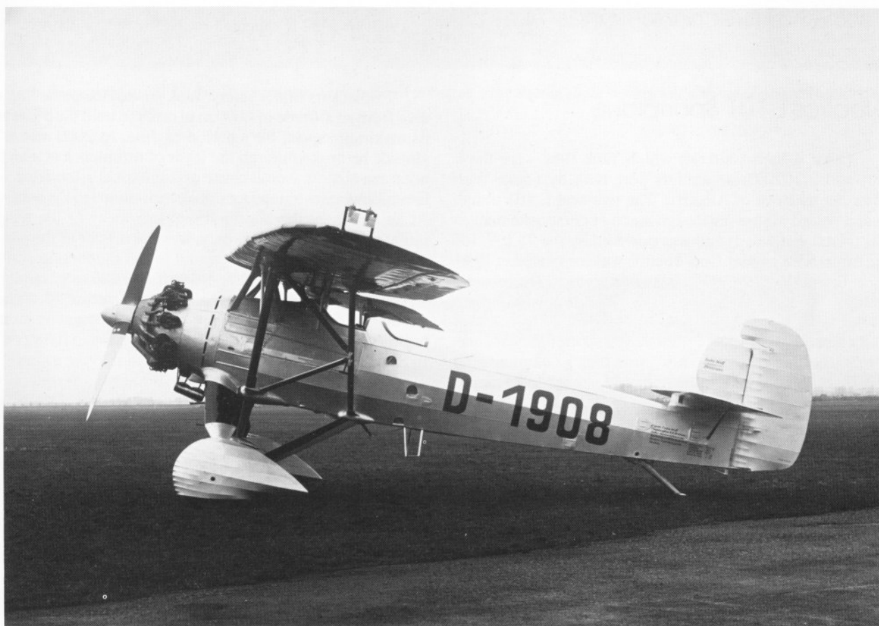
Fw 40 (A 40) with an uncowled Jupiter engine. It later served as a weather reconnaissance aircraft.
