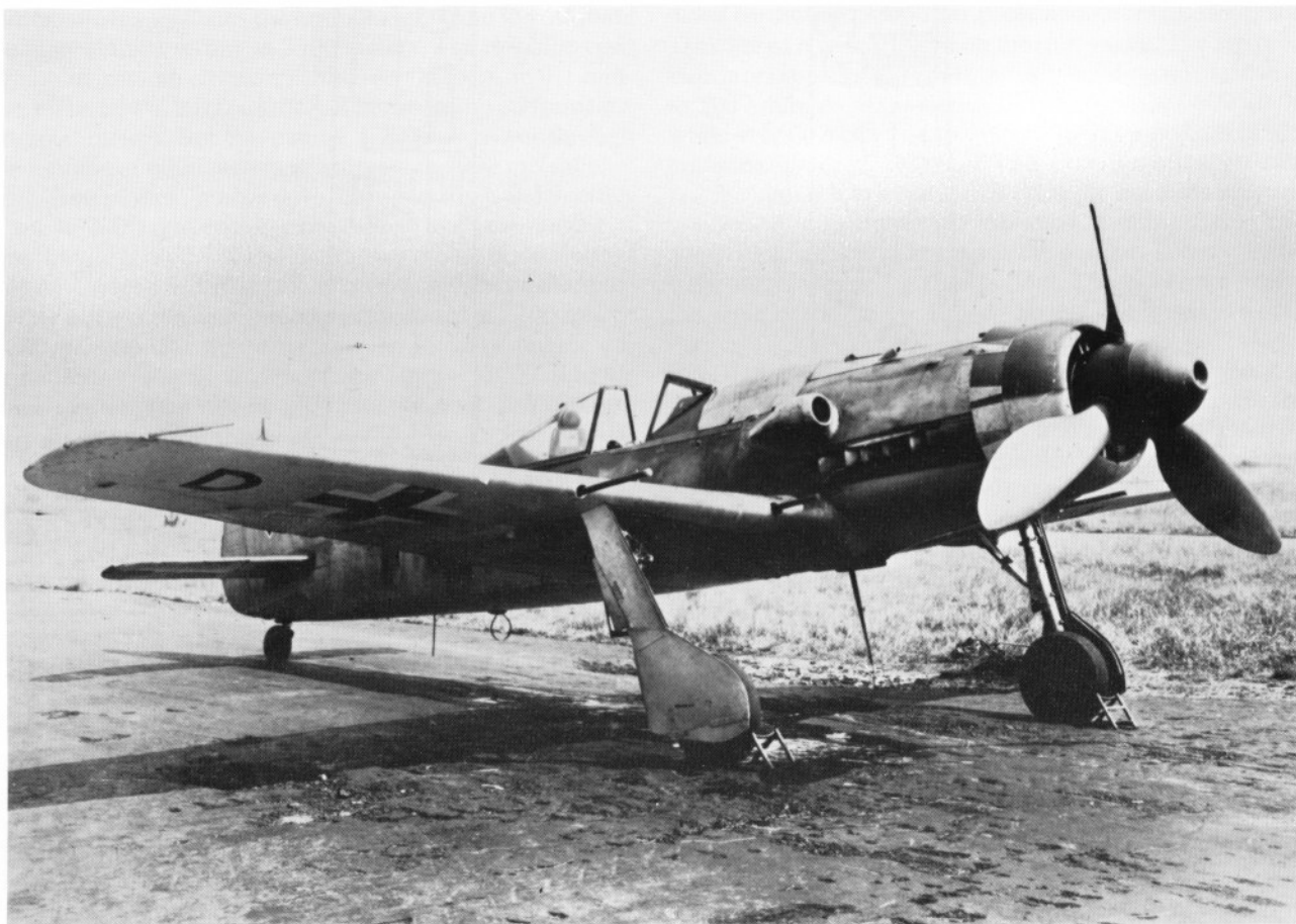
The Fw 190D-11 strike fighter with Jumo 213F and a 30-mm Mk 108 cannon firing through the propeller hub.
