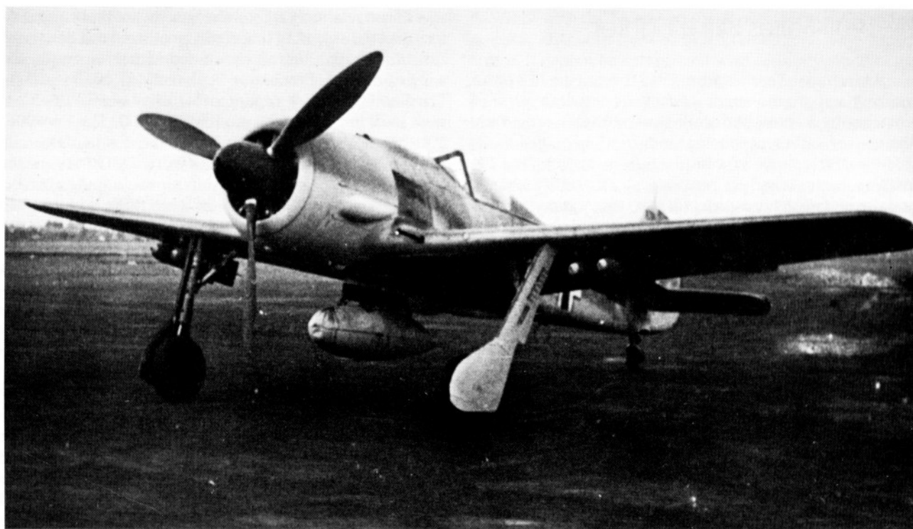
Fw 190F-8/R1 with 300-l auxiliary fuel tank under the fuselage and two ETC 50 racks under each wing, each holding a 50-kg bomb.
