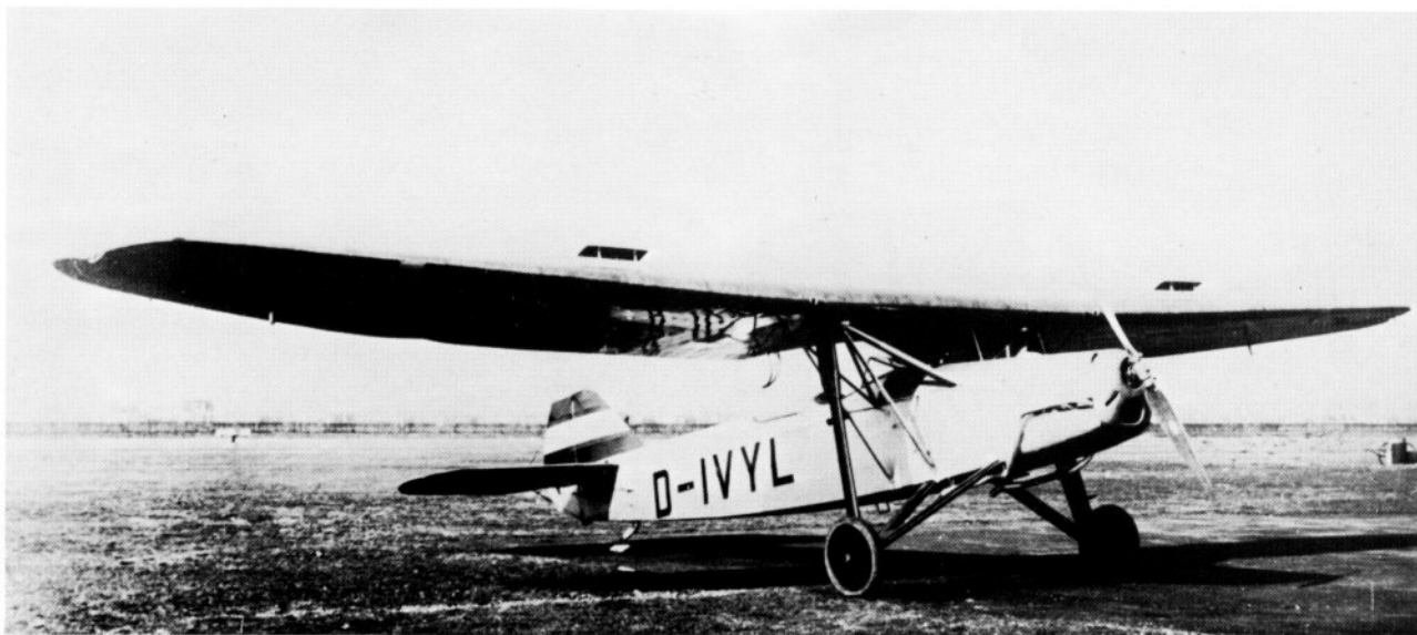
Focke-Wulf Fw 47C, a specialized weather reconnaissance aircraft powered by an Argus As 10C engine with 176 kW (240 hp), first built in 1932. The meteorologists gave the airplane the nickname of "Höhengeier" (Alpine buzzard).
