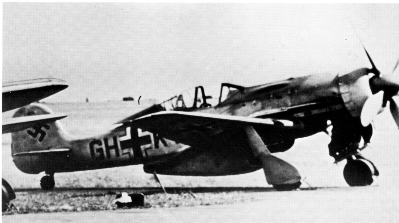
Fw 190 V30 GH+KT Kängeruh with DB 603S, TK 11 turbo-supercharger and pressurized cockpit. The aircraft was later fitted with the Jumo 213E and subsequently served as the prototype for the H-0 series.
