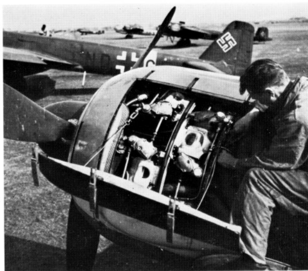
The BMW 801D was easily accessible thanks to its fold-down shroud covers.
