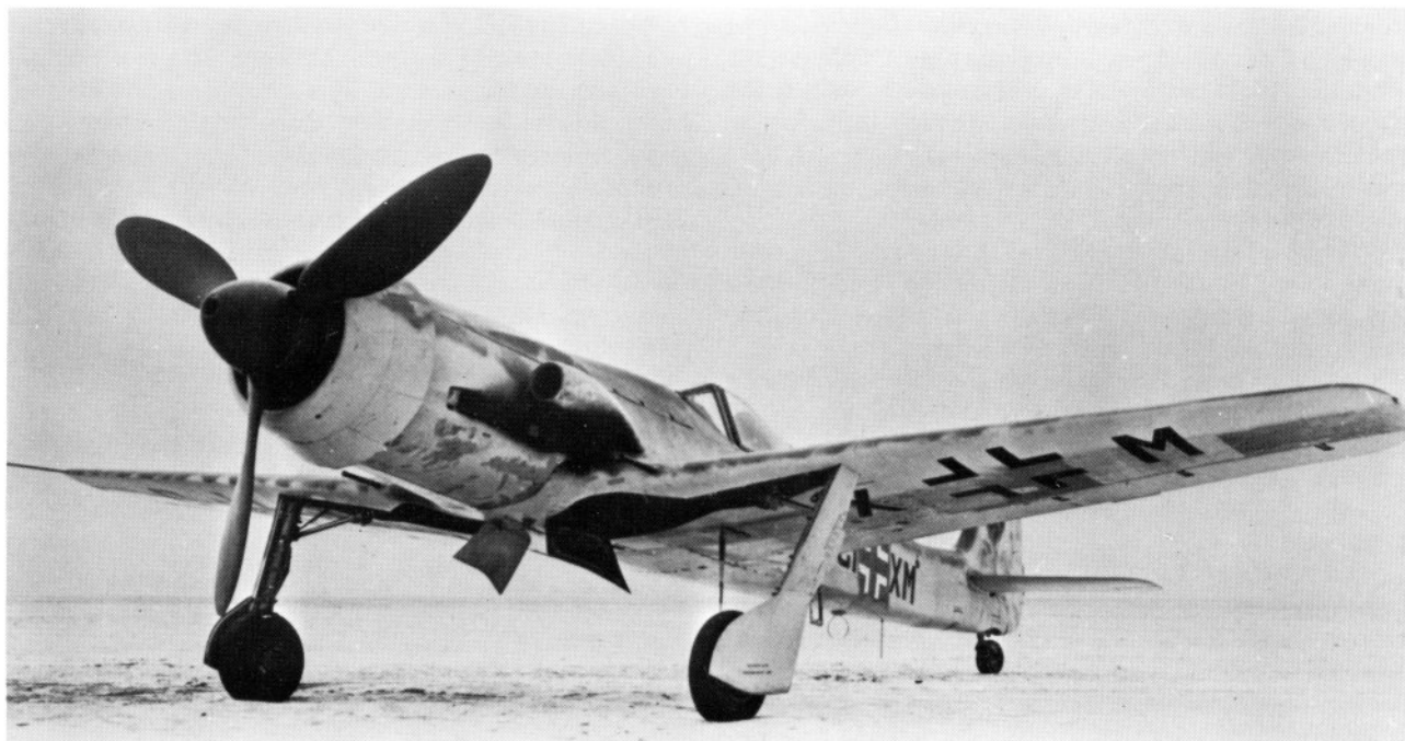
The Ta 152 V7 with Werknummer 110007 was built in Cottbus and became the prototype for the Ta 152 C-0/R11 with DB 603L engine and MW 50 injection. It was expected to enter production in March of 1945.
