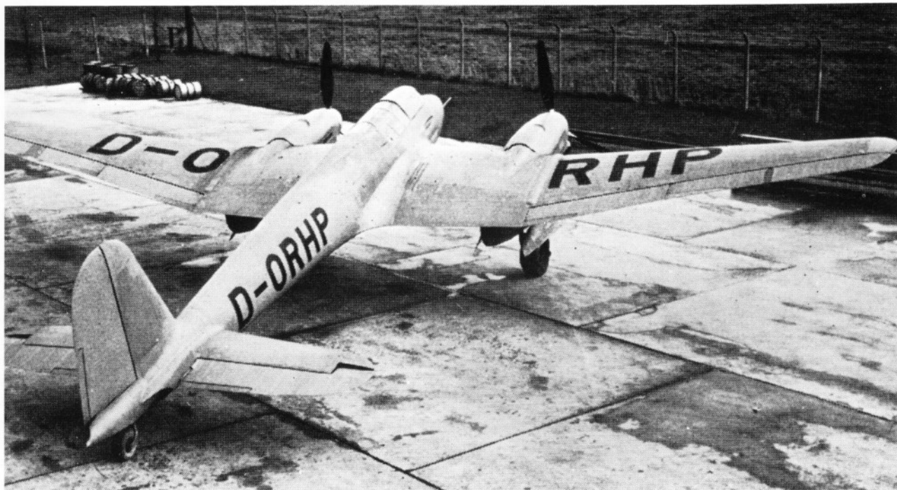
During the assembly process the Fw 187 V3 was converted into a two-seat "Zerstörer" attack plane.
