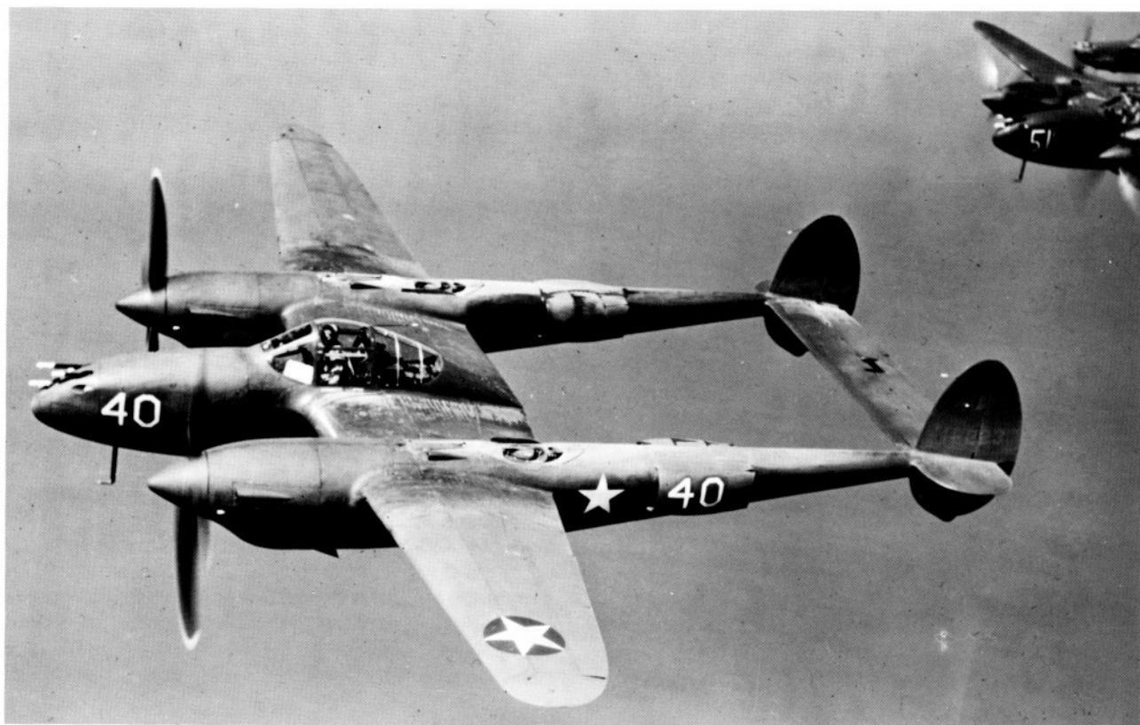
Lockheed P-38F Lightning with two Allison V-1710-49/53 engines, year of service 1942.
