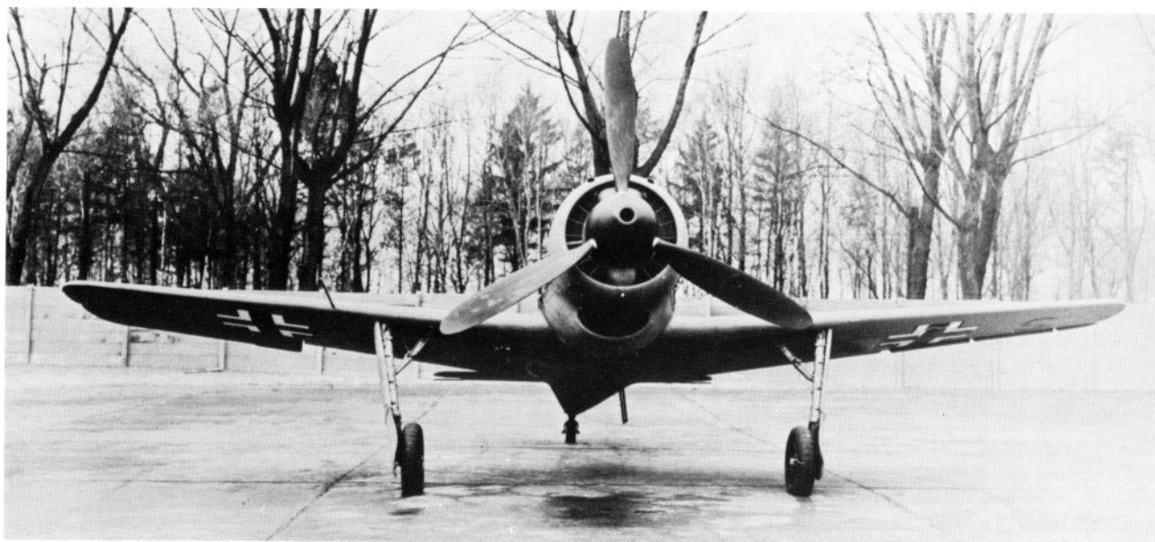
Fw 190C V13 with DB 603A and belly oil cooler.
