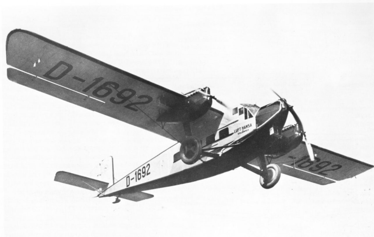
Rohrbach Ro VIII Roland II with three 265 kW (360 hp) BMW Va engines and having an enclosed cockpit with the side panes of the canopy set quite low down on the fuselage nose.
