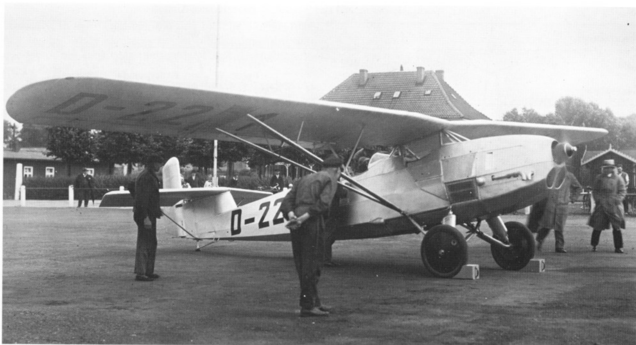
While flying the AL 102 L (Fw 55 L) trainer, Tank suffered a broken wing during flight testing when the plane began oscillating violently during landing.
