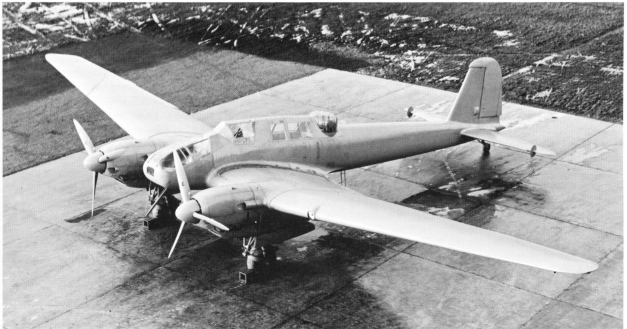
The Fw 57 with DB 600C engines. This prototype was Focke-Wulf's first all-metal aircraft design, a new role for Tank's engineering and assembly team.
