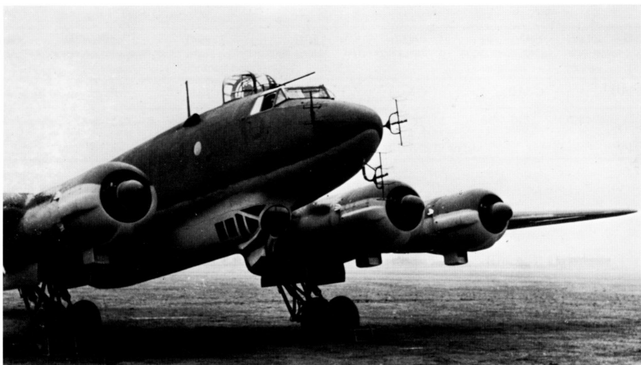
Fw 200C-6 with the latest radar systems designed for searching out submarines.
