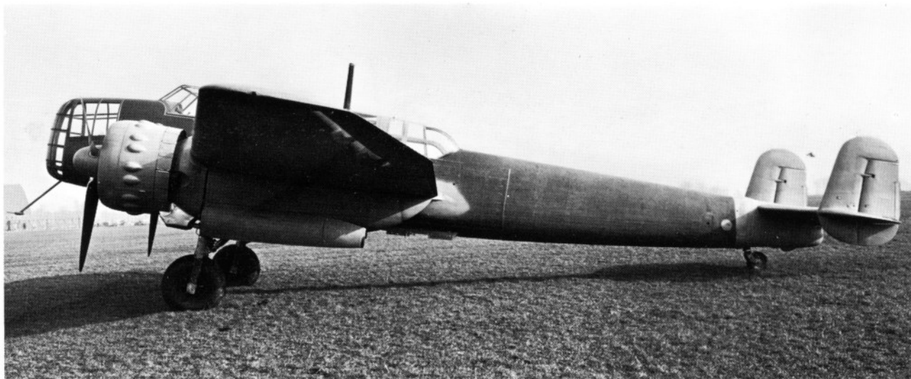
The Henschel Hs 124 V2, with air-cooled BMW 132 Dc engines, was a direct competitor of the Fw 57.
