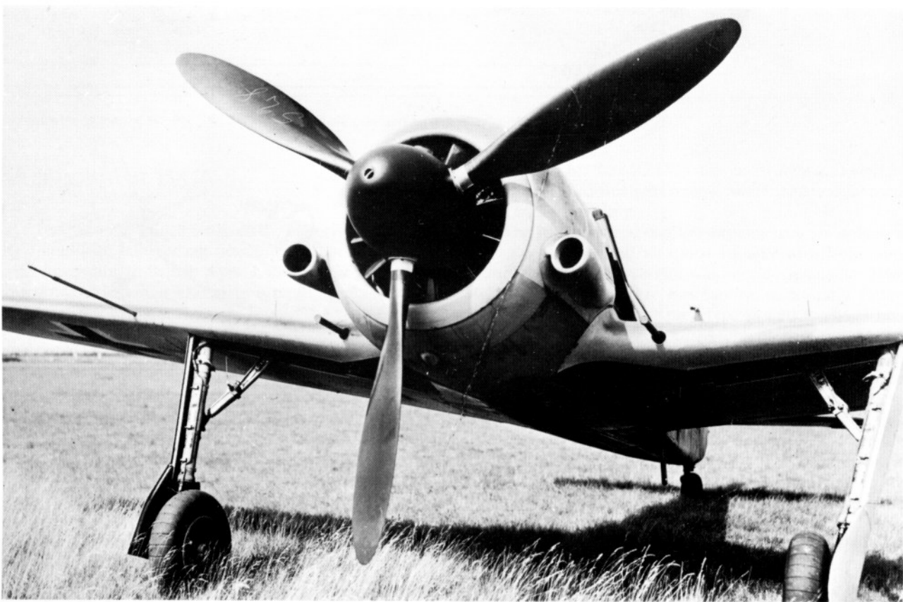
Fw 190A-3/U7 with BMW 801D and intake filters for operations in tropical climates.
