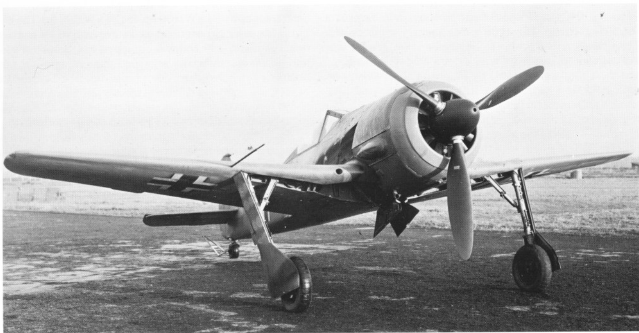
Fw 190 V5K, the fifth prototype here with the original short wings, was the first one to be fitted with the more powerful BMW 801 C-0 engine (with an output of 1147 kW/1560 hp)
