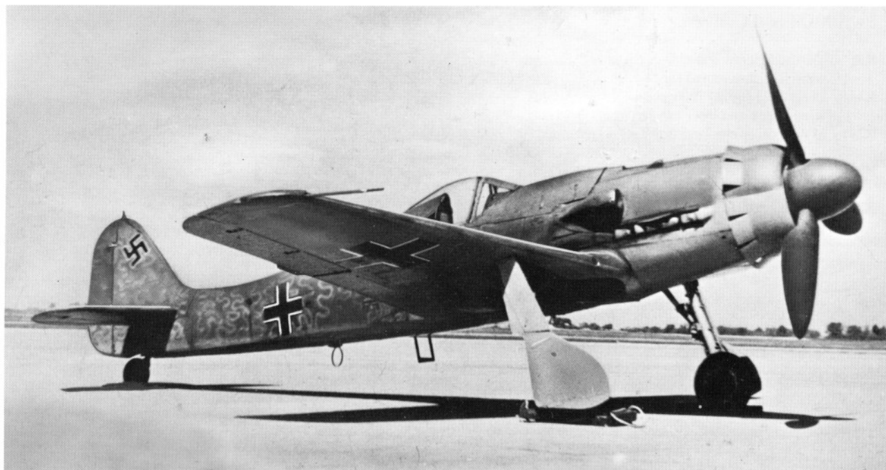
The Fw 190D-9 revealed a new single-piece blown canopy and was fitted with the Jumo 213A.
