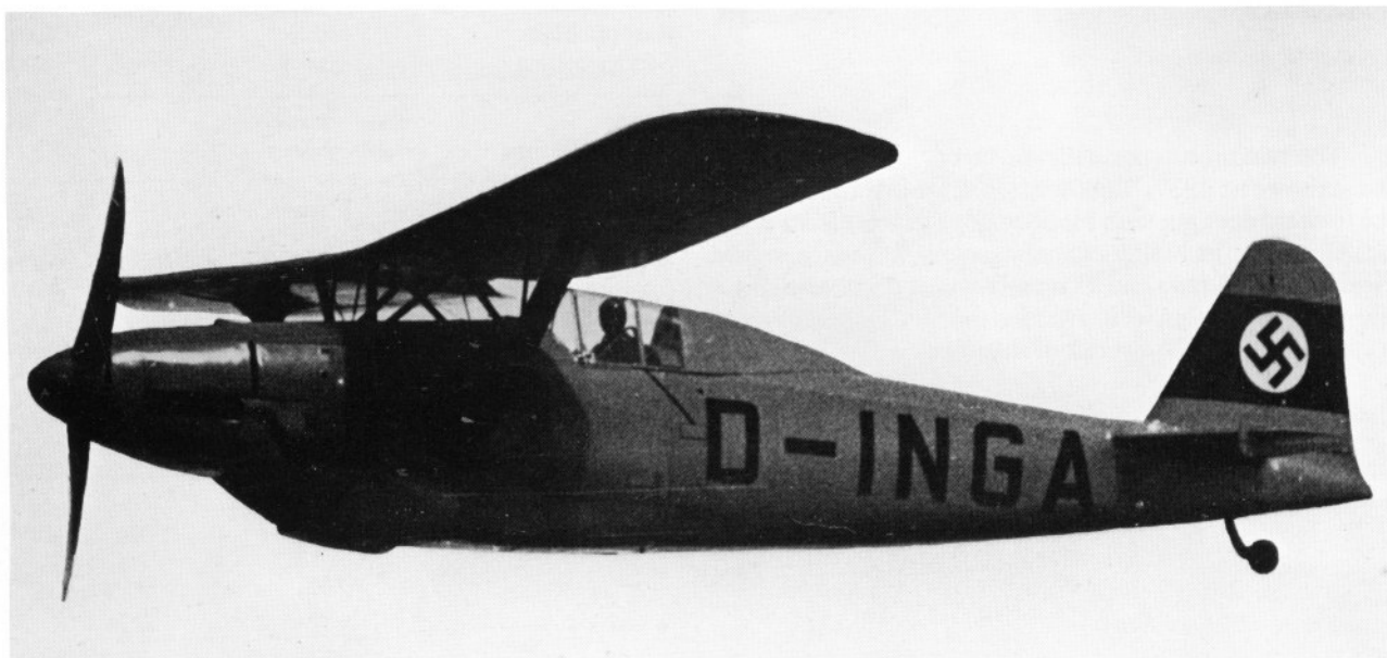
Fw 159 V2 fighter plane. Utilizing a variable-pitch propeller, the aircraft could reach speeds of 385 km/h at 4500 meters.
