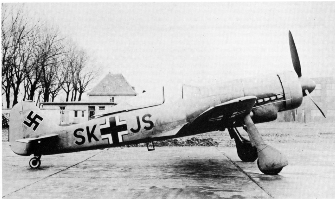
Fw 190 V13 engine testbed for the DB 603A (Werknummer 0036). First prototype of the Fw 190C series.
