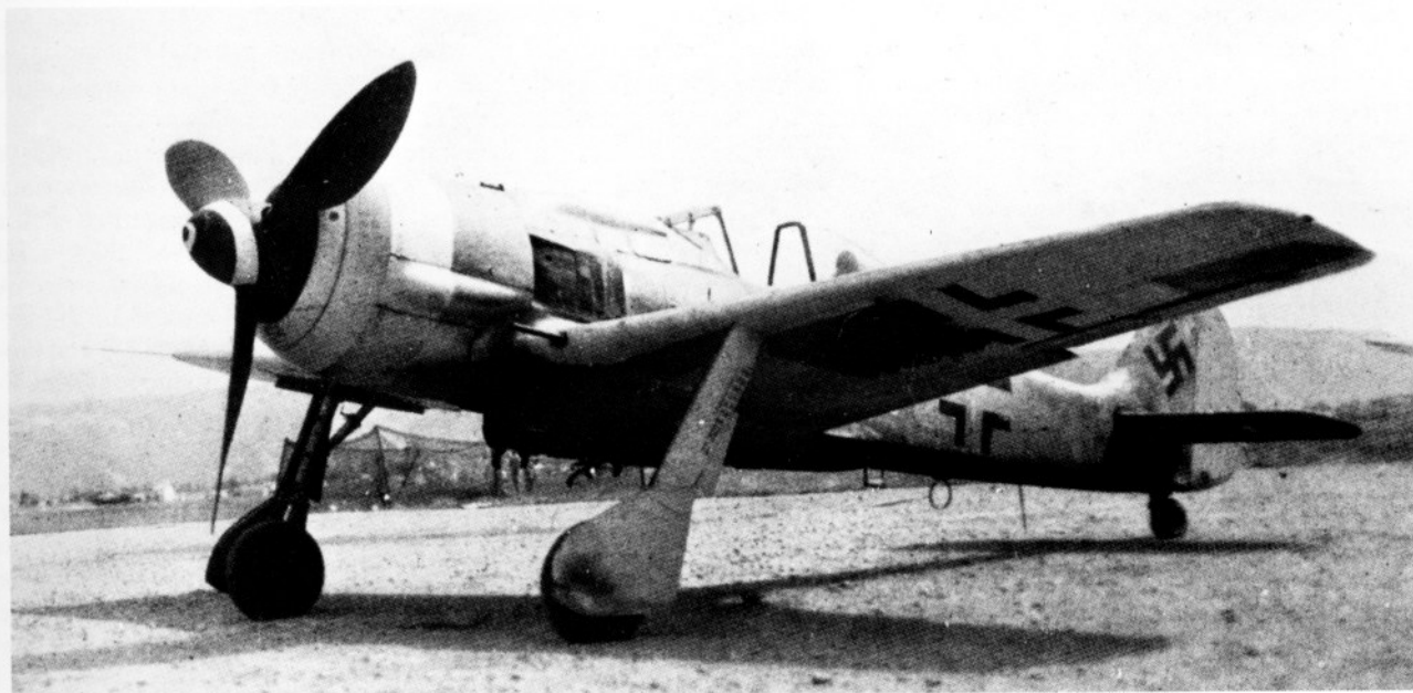
The wings of the Fw 190F-8 ground attack variant were reinforced in the area of the landing gear. This aircraft was used in the Mediterranean theater.
