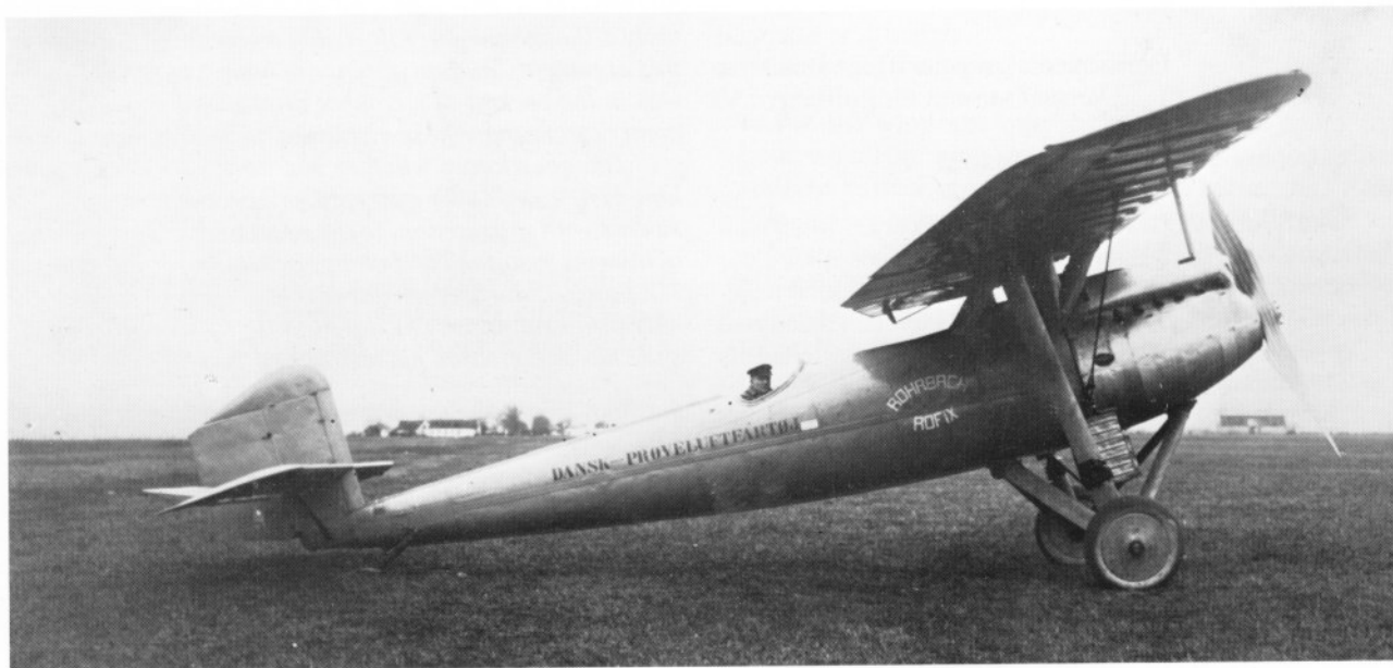
The Rohrbach Ro IX Rofix V 2 single seat fighter. The wings - at least as they appear in the photo - no longer seem to have any dihedral. This is therefore probably the second prototype, Werknummer 23, in which Paul Bäumer crashed.
