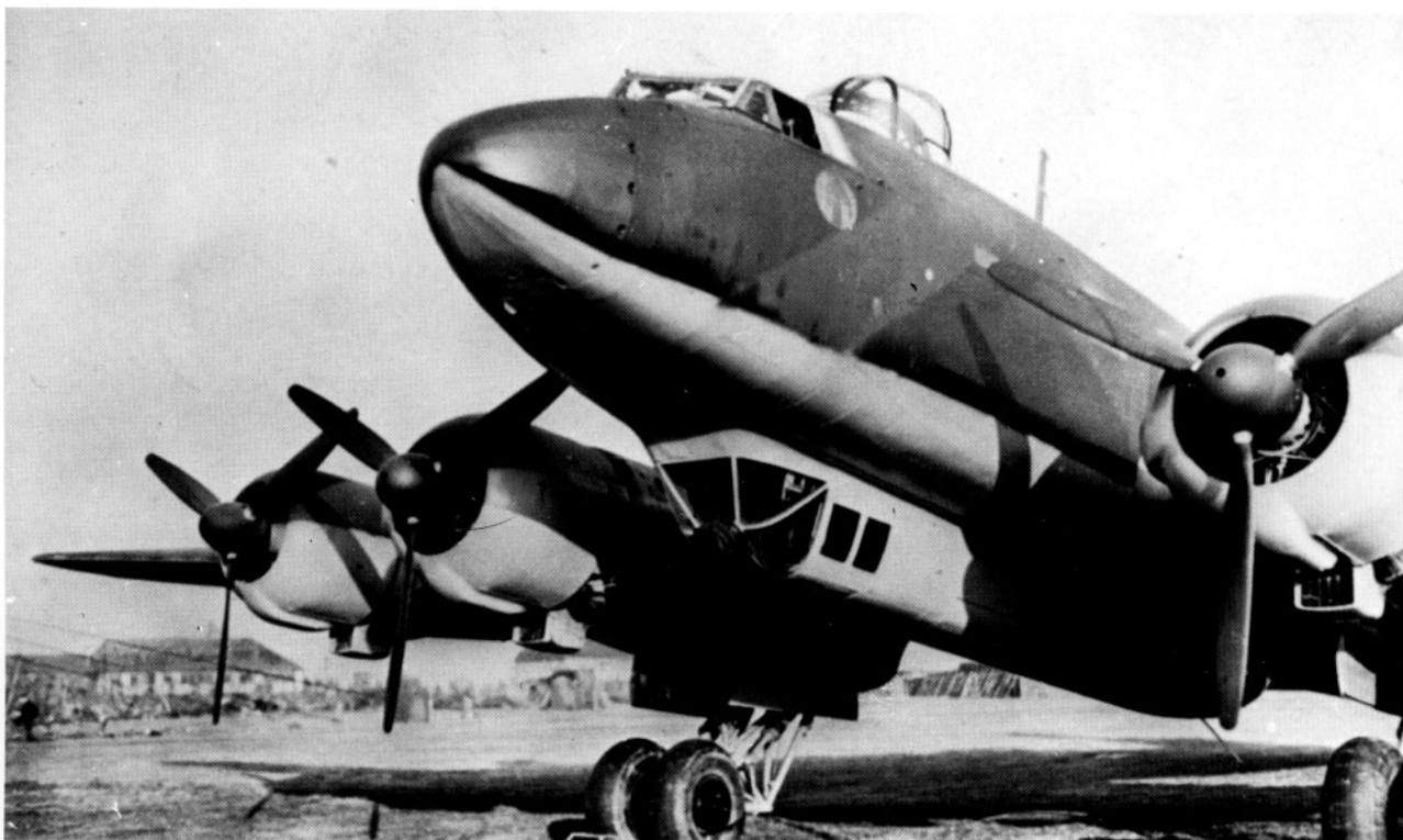
Fw 200C-4 with added armament, year of service 1942.
