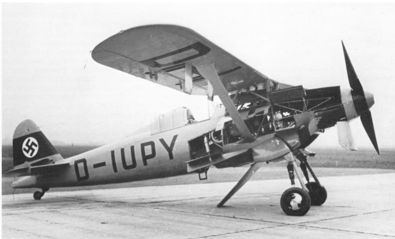
Fw 159 V3 during flight testing, seen with its cover plates removed.
