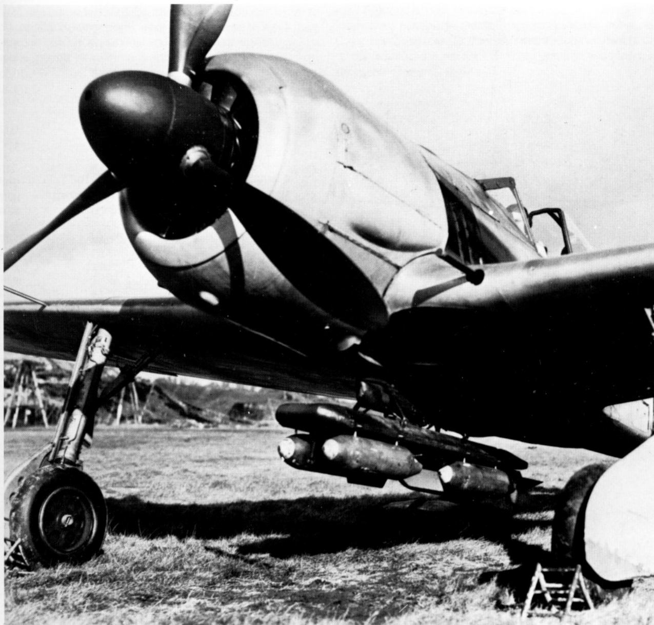
Fw 190G-8 with ETC 501 and ER 4 rack holding four 50-kg bombs.
