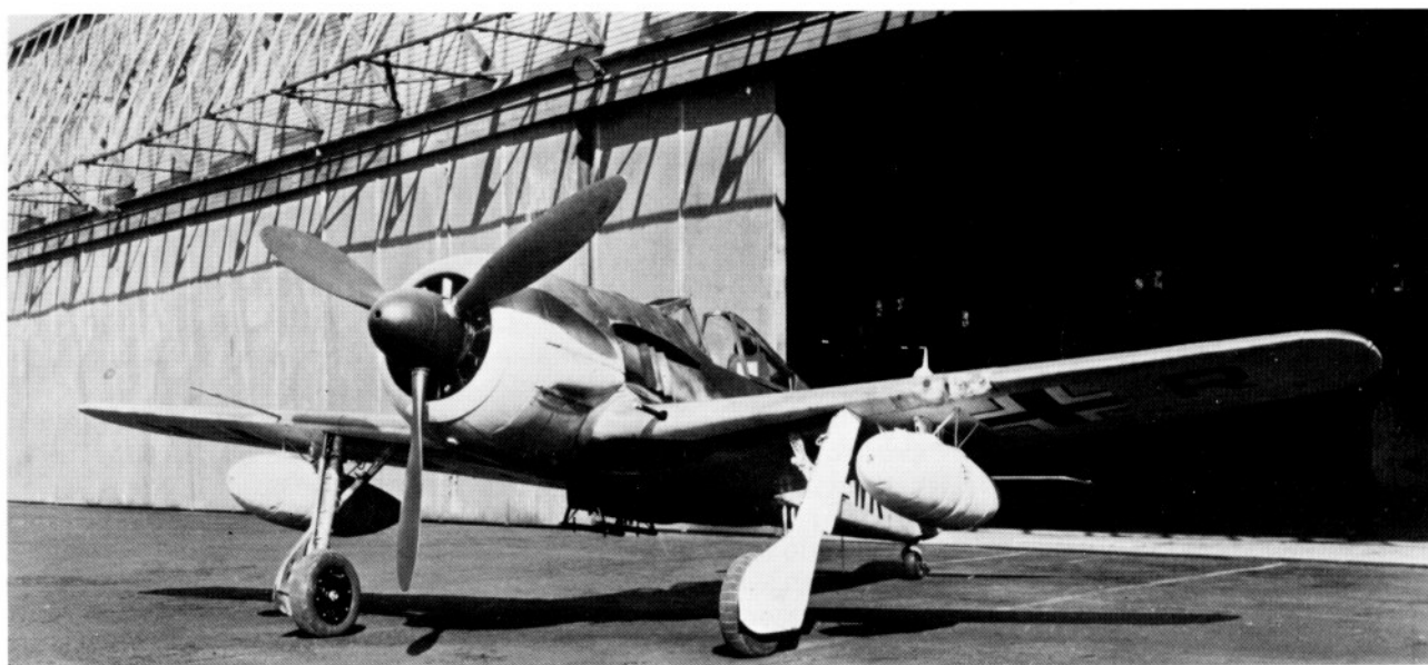
Fw 190A-5/U2 with auxiliary tanks and flash guards for night fighting operations.
