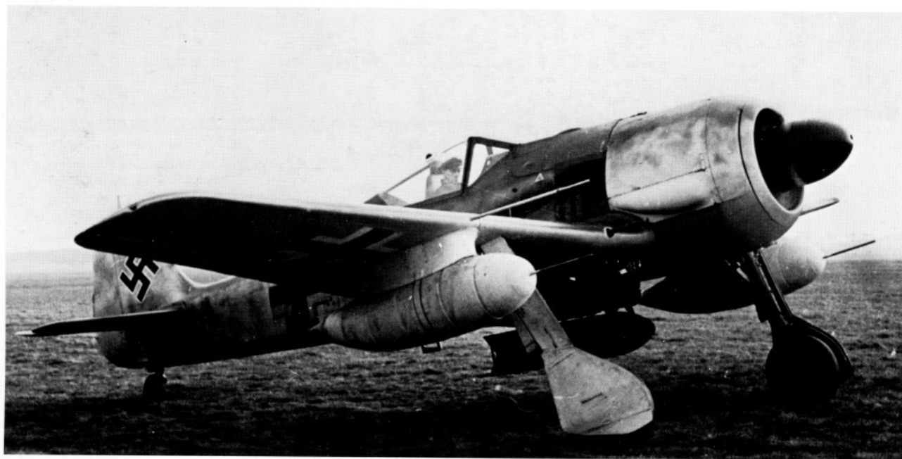
Fw 190G-3 long-range fighter-bomber with 500-kg bomb and two 300-l auxiliary fuel tanks, year of service 1944.
